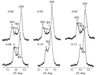
Fig. 1. Fragments of diffraction patterns of SS of the studied system. Values near the curves represent concentration of Sr  $(\alpha_1)$  in arb. units.
