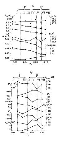
Fig. 2. Relationships of densities, structural (*a*) and electrophysical (*b*) parameters studied for SS for concentration Sr  $(\alpha_1)$ : 1- *a*, 2- *c*/*a*, 3- *c*, 4-V, 5, 6, 7- densities experimental, X-Ray and relative, respectively.
