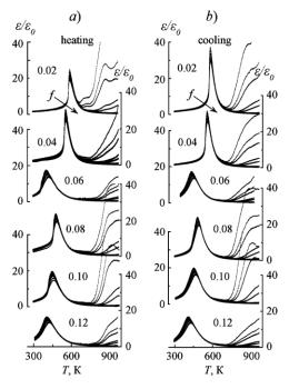
Fig. 3. Dielectric spectra of SS of the studied system in heating mode (*a*) and cooling mode (*b*). Numbers near the curves represent concentration of Sr ( $\alpha_1$ ) in arb. units.
